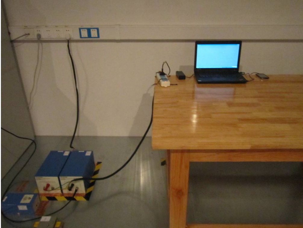
Conducted Emissions Test Setup Front View
