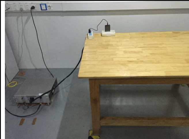
Conducted Emissions Test Setup Front View
