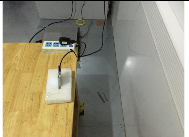
Conducted Emissions Test Setup Side View
