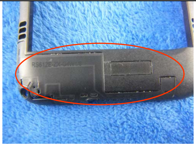
GSM/PCS/UMTS-FDD Antenna View
