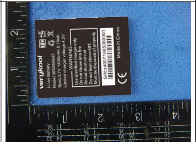
Battery - Rear View
