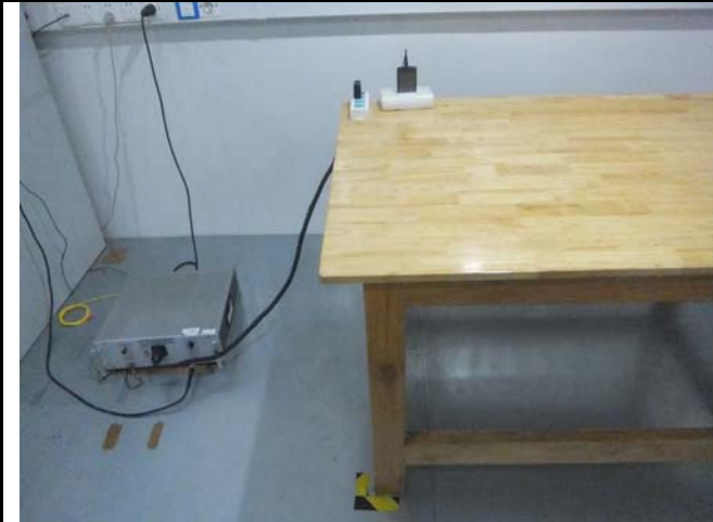
Conducted Emissions Test Setup Front View
