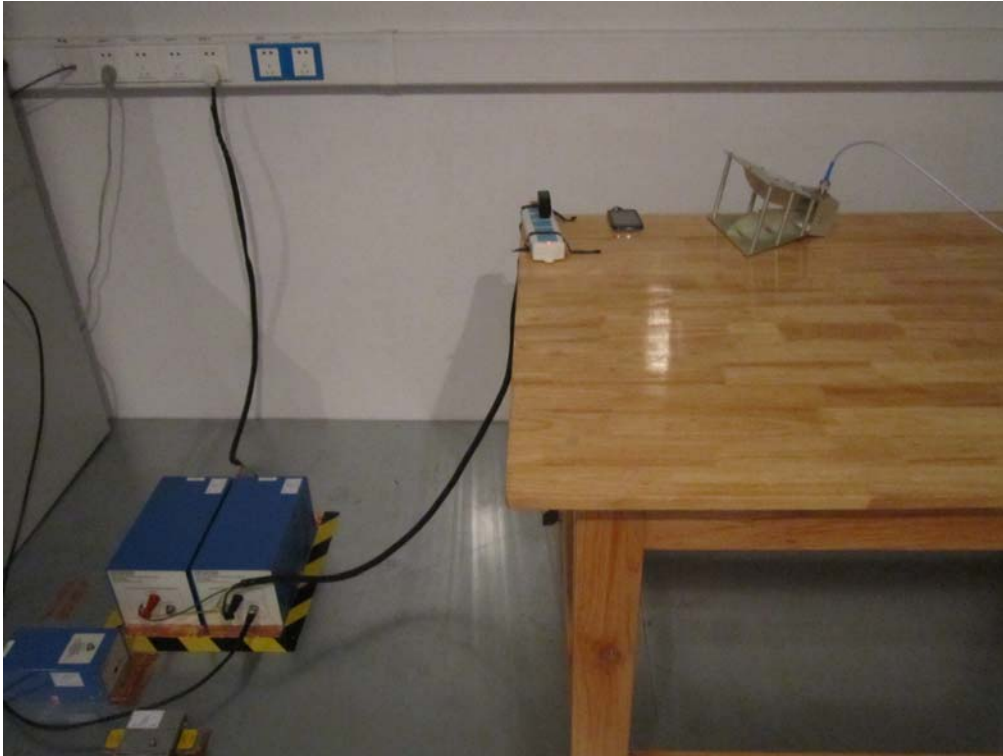
Conducted Emissions Test Setup Front View
