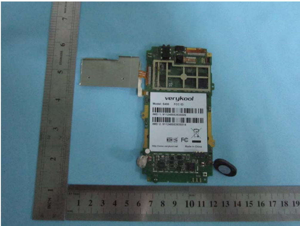
Mainboard Without Shielding - Bottom View
