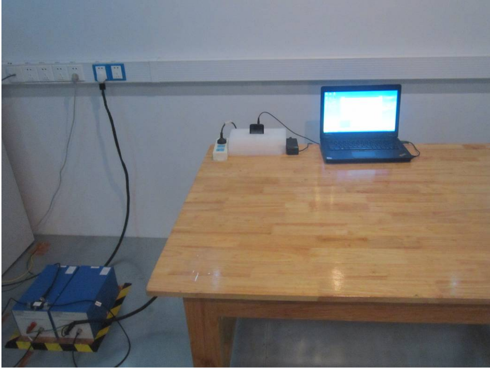
Conducted Emissions Test Setup Front View
