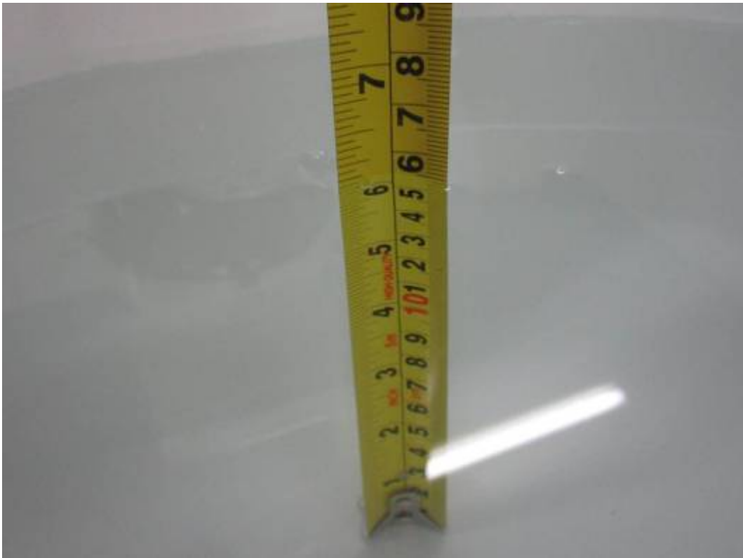
Liquid depth \geq 15cm
