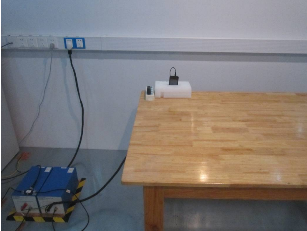
Conducted Emissions Test Setup Front View
