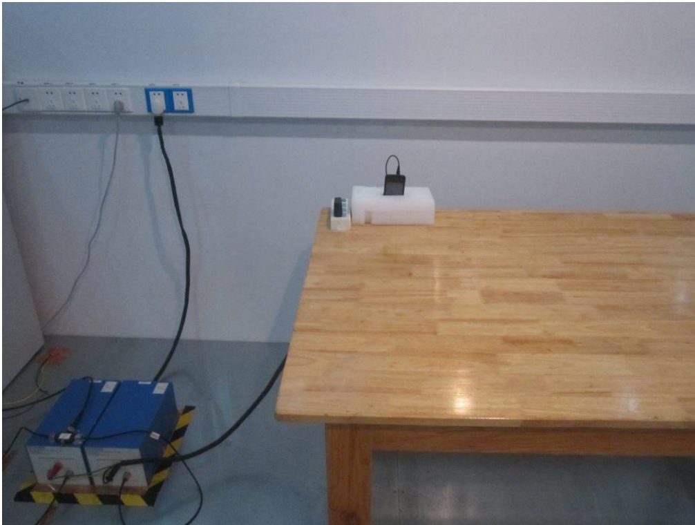
Conducted Emissions Test Setup Front View
