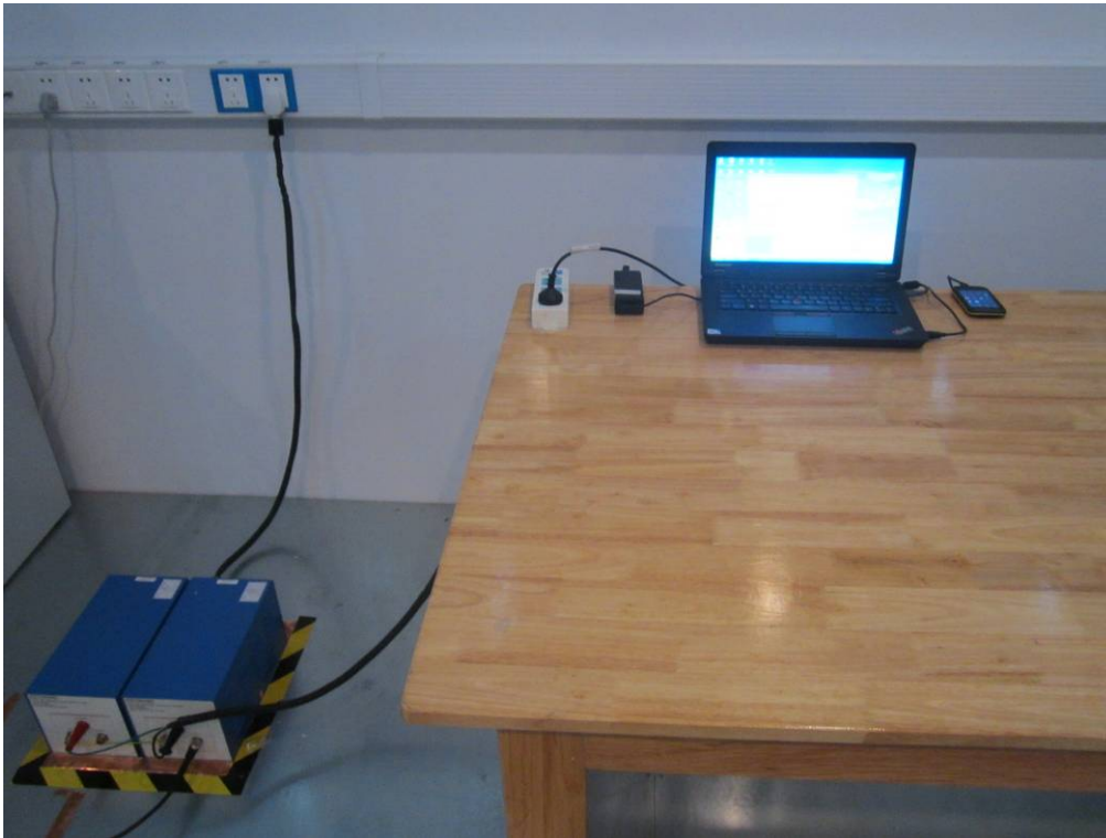
Conducted Emissions Test Setup Front View
