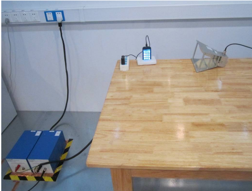
Conducted Emissions Test Setup Front View
