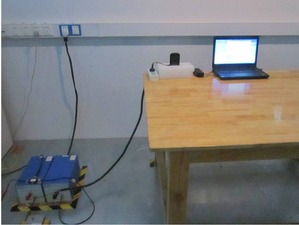
Conducted Emissions Test Setup Front View
