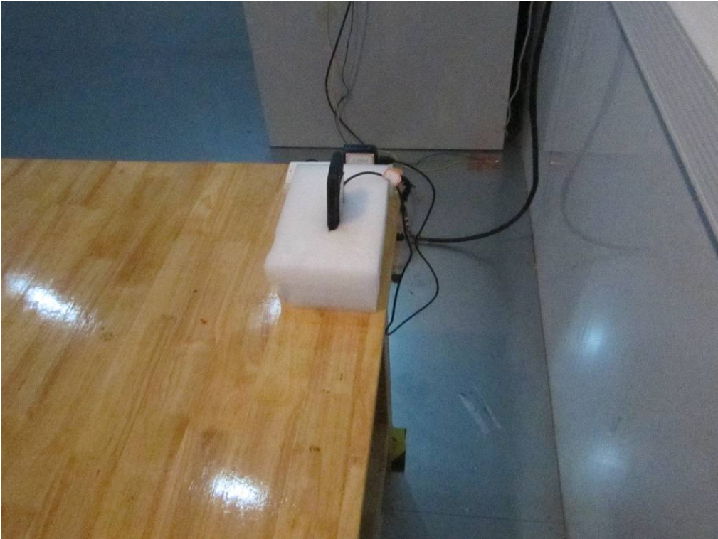
Conducted Emissions Test Setup Side View
