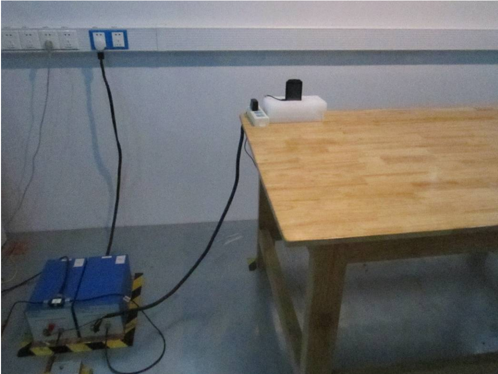
Conducted Emissions Test Setup Front View
