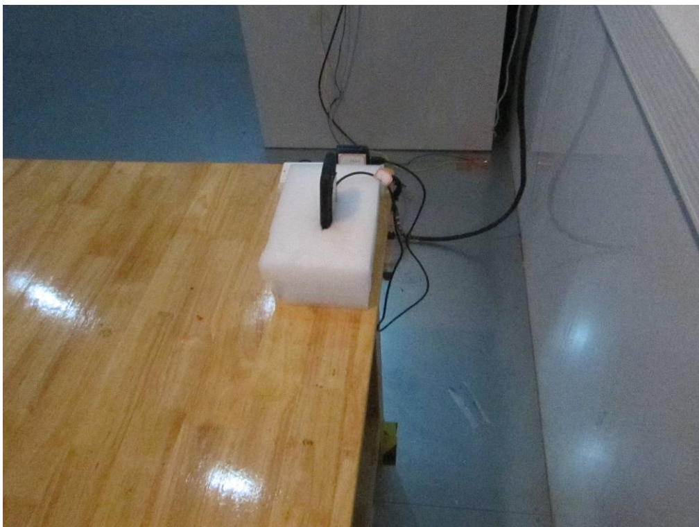
Conducted Emissions Test Setup Side View
