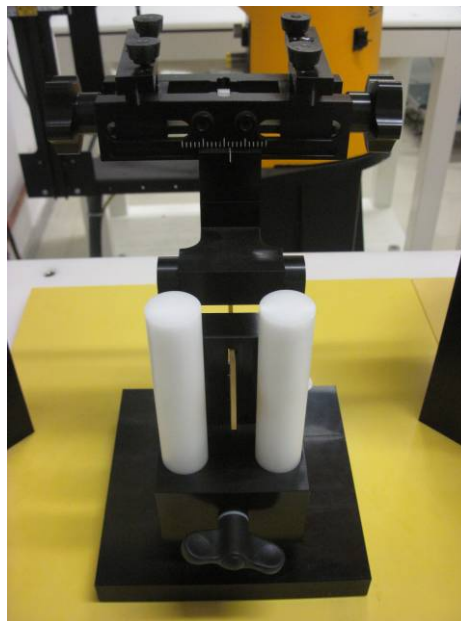
Figure 6.4 HAC Phantom & Device Holder
