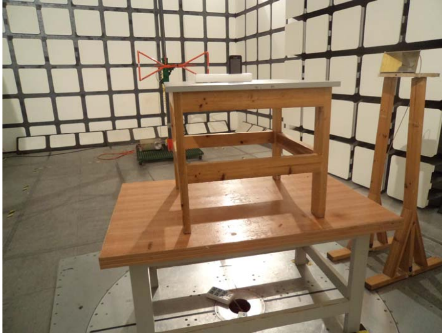
Radiated Emissions Test View (Below 1 GHz)
