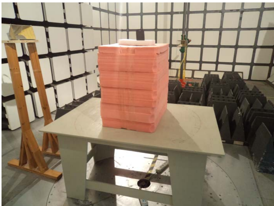
Radiated Emissions Test View (Above 1 GHz)
