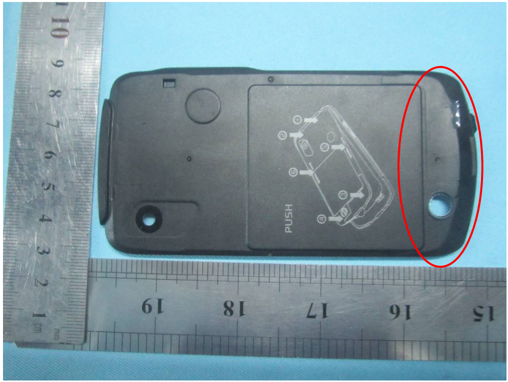
GSM/UMTS Antenna View
