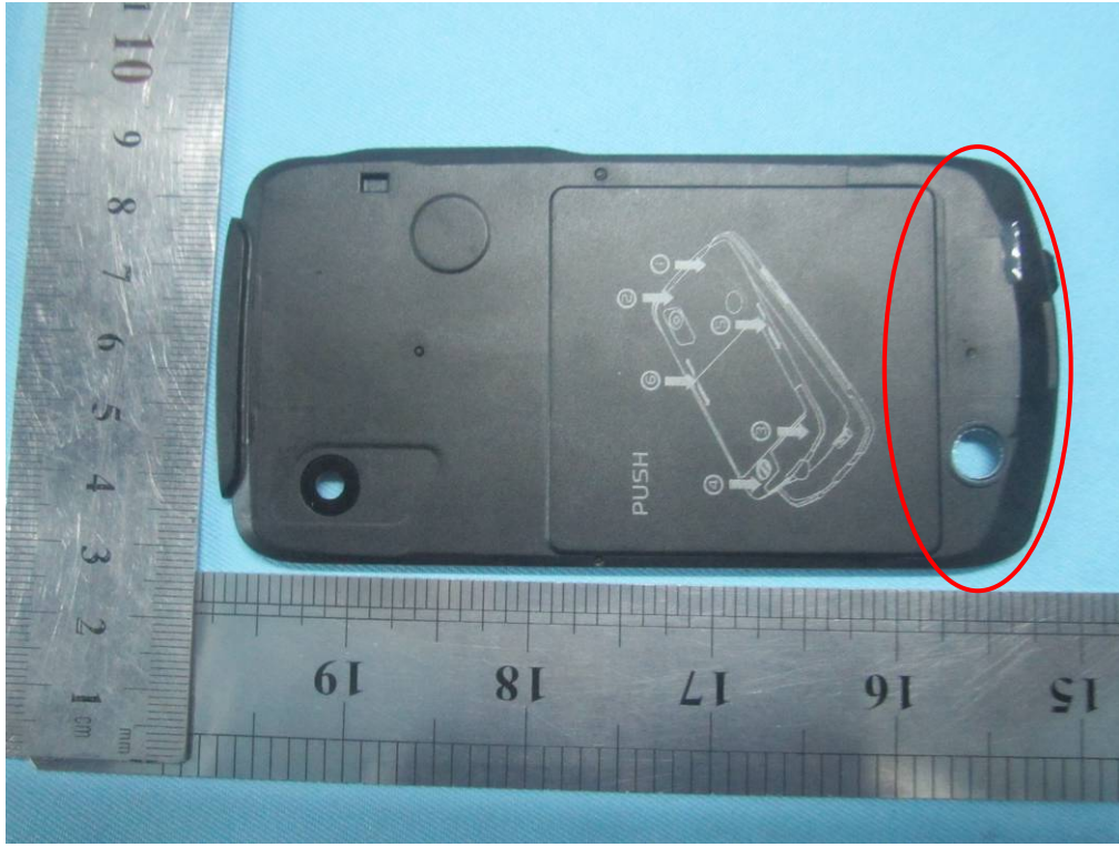
GSM/UMTS Antenna View
