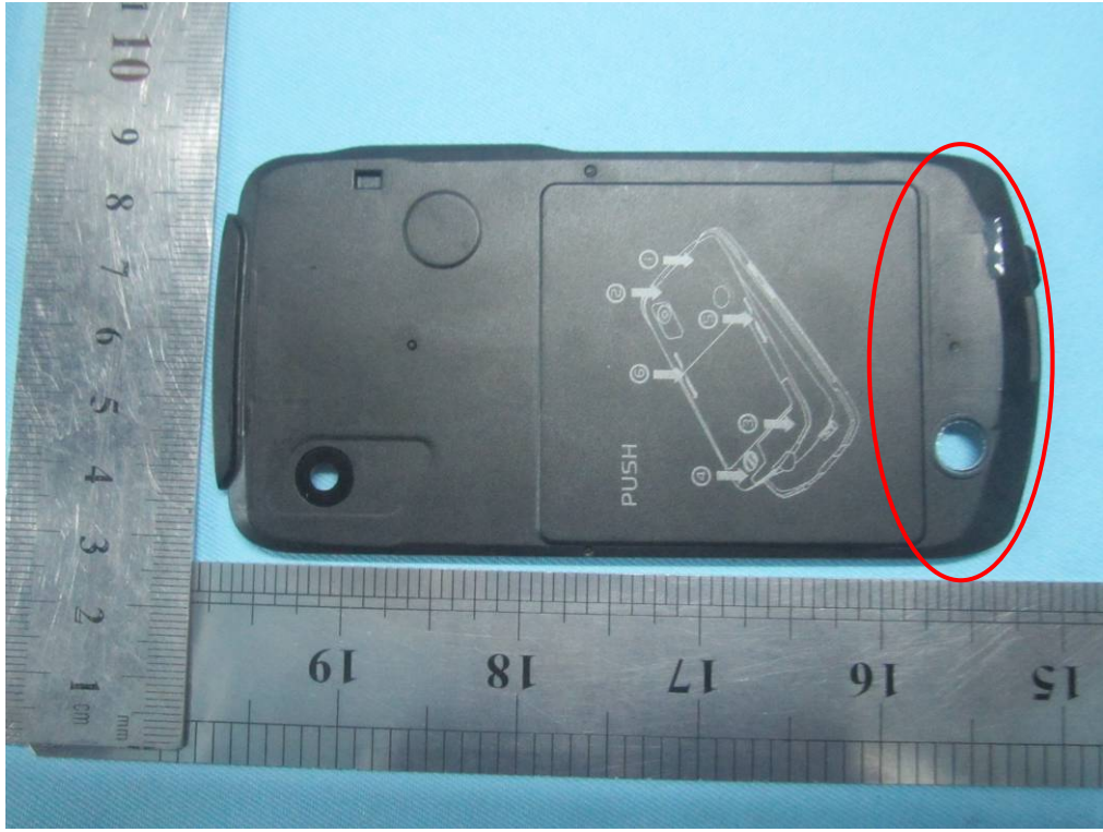
GSM/UMTS Antenna View
