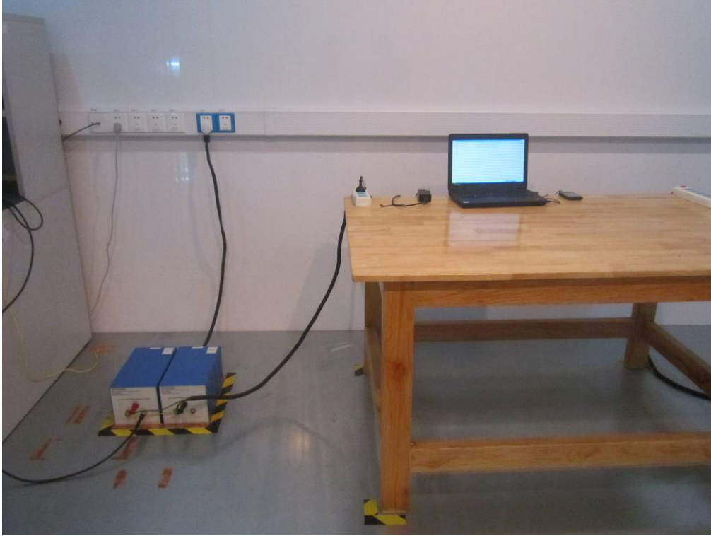
Conducted Emissions Test Setup Front View
