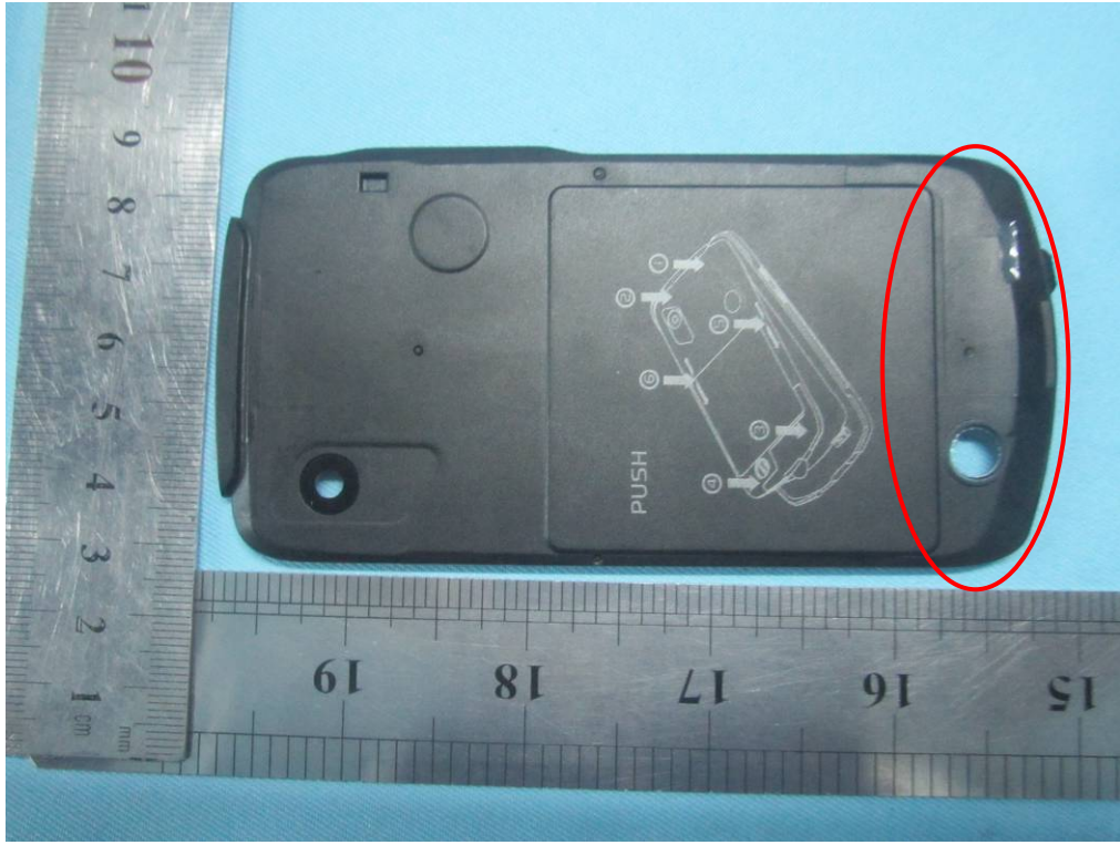
GSM/UMTS Antenna View
