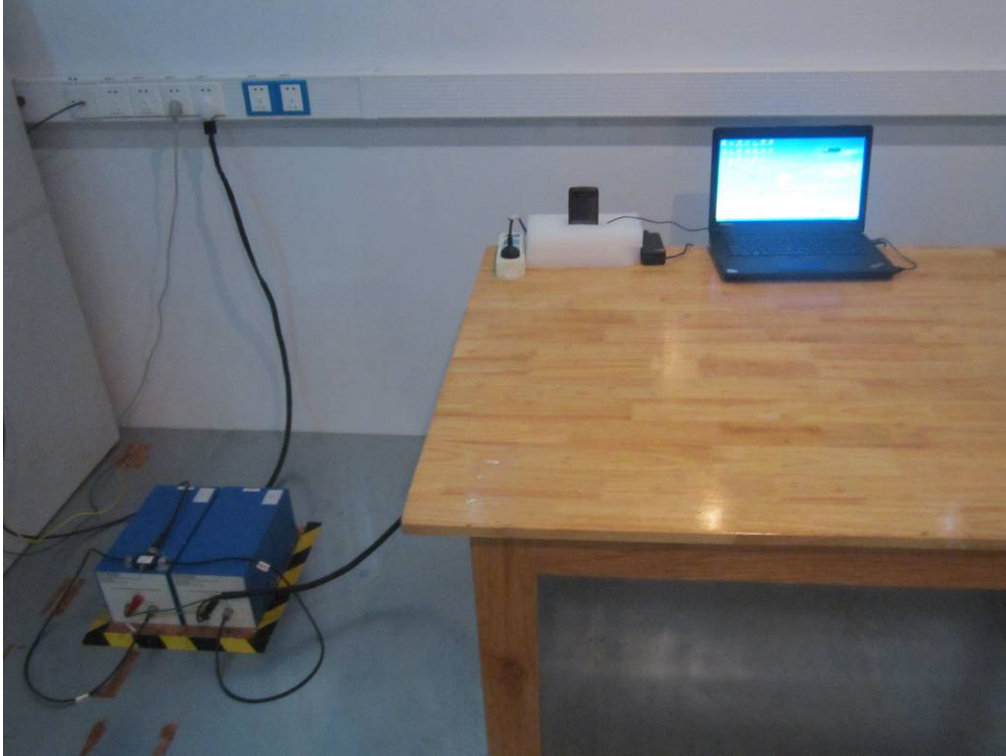
Conducted Emissions Test Setup Front View
