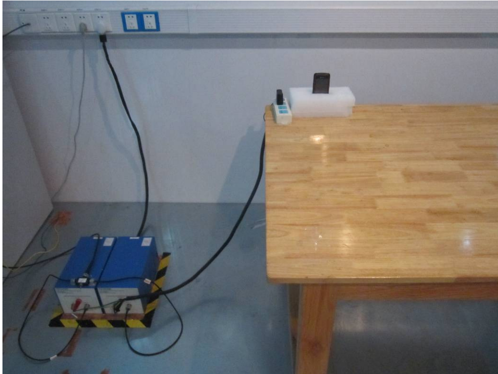
Conducted Emissions Test Setup Front View
