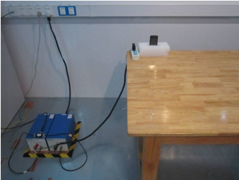
Conducted Emissions Test Setup Front View
