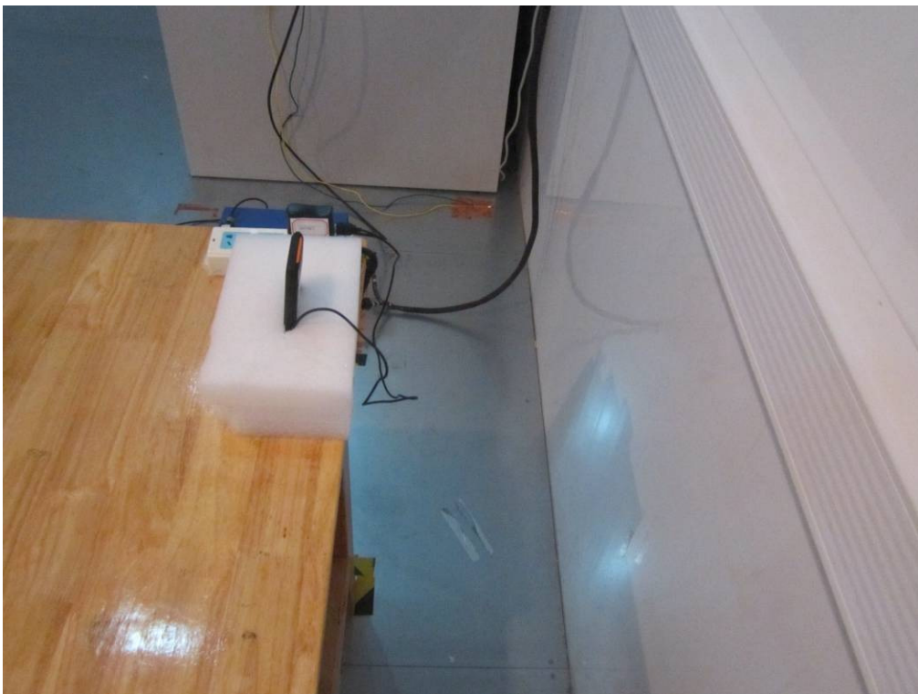
Conducted Emissions Test Setup Side View
