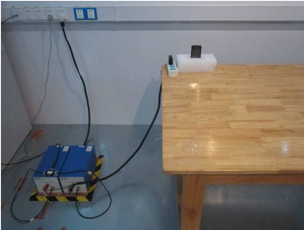
Conducted Emissions Test Setup Front View
