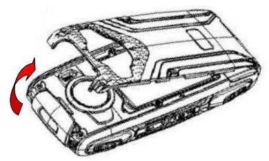
■ Dig out the bottom of the battery and get the battery out.
