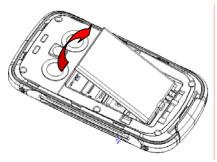
■ When installing the battery, insert the metal teeth at the bottom of the battery into corresponding slot of the mobile phone, and then press the battery down to install the battery in place. The battery must be ensured to be installed before power on.
