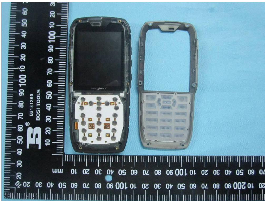
Cover Off - Front Housing View
