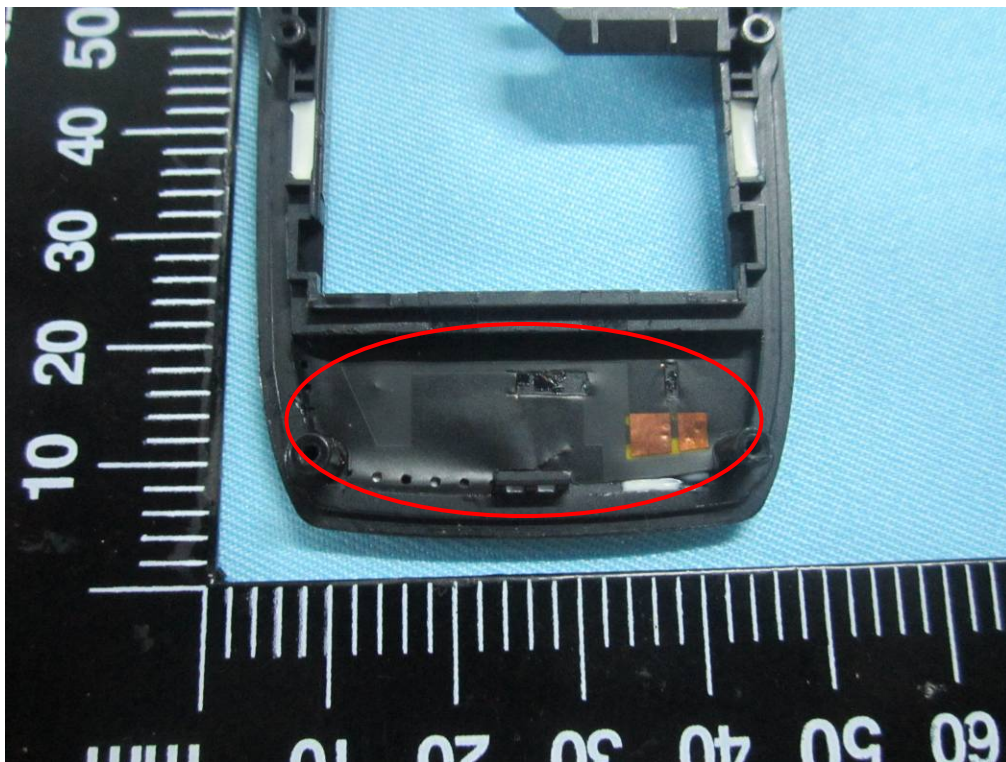
GSM / UMTS - Antenna View
