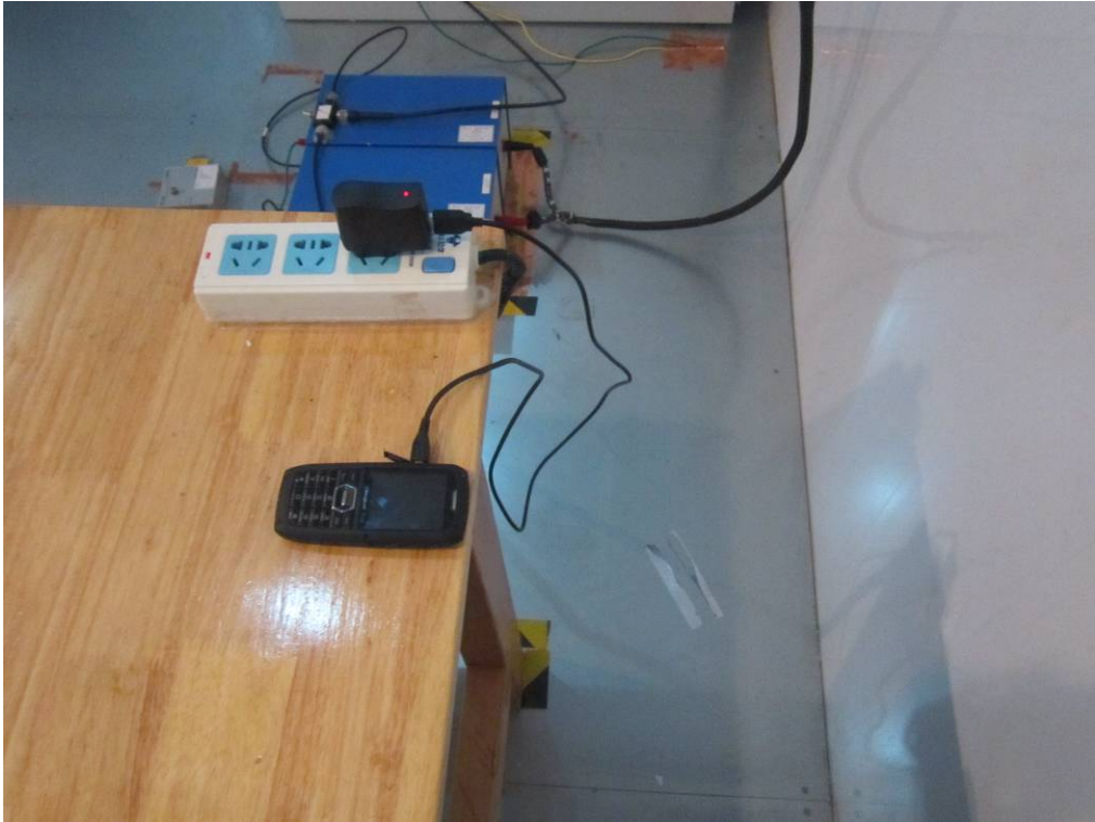
Conducted Emissions Test Setup Side View
