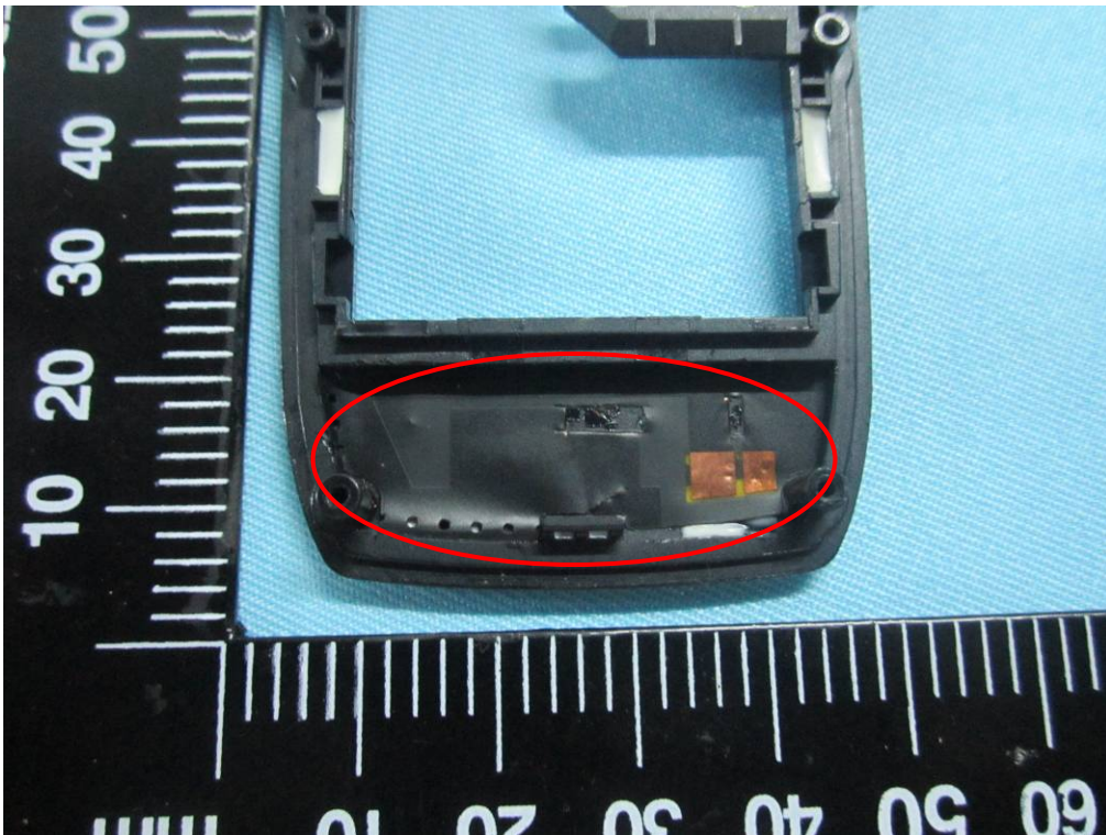
GSM / UMTS - Antenna View
