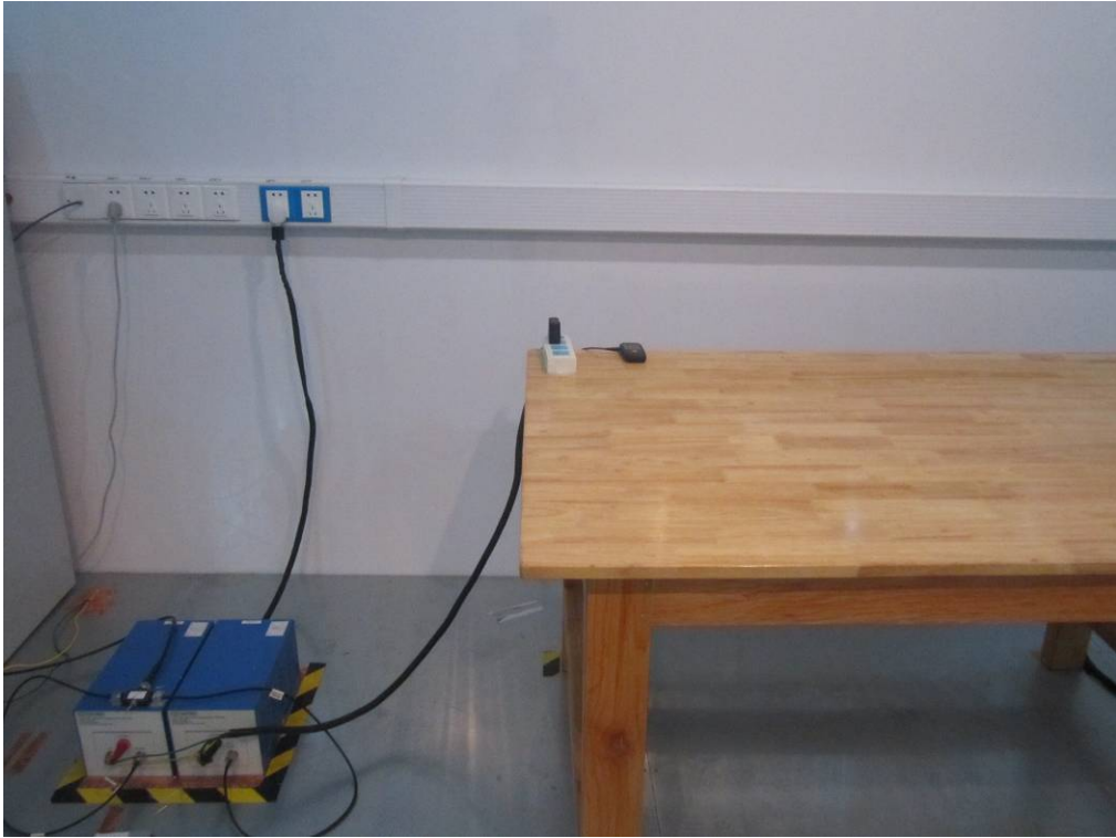
Conducted Emissions Test Setup Front View
