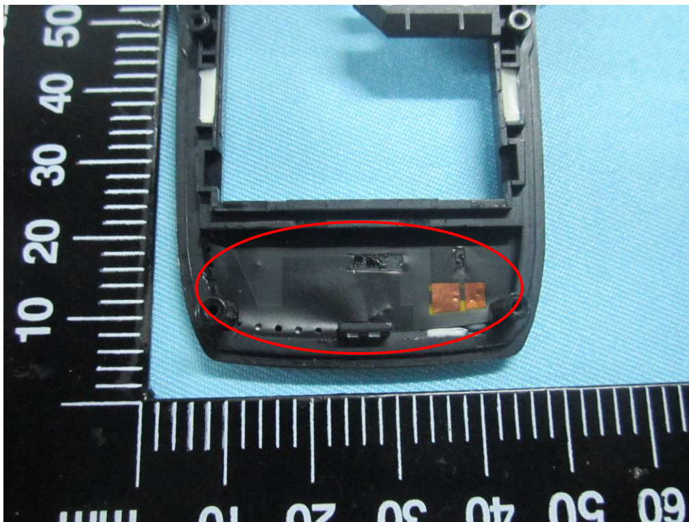
GSM / UMTS - Antenna View
