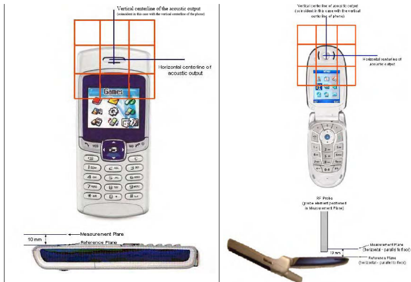
Figure 1. WD reference and plan for RF emission measurement
