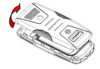
Dig out the bottom of the battery and get the battery out.
