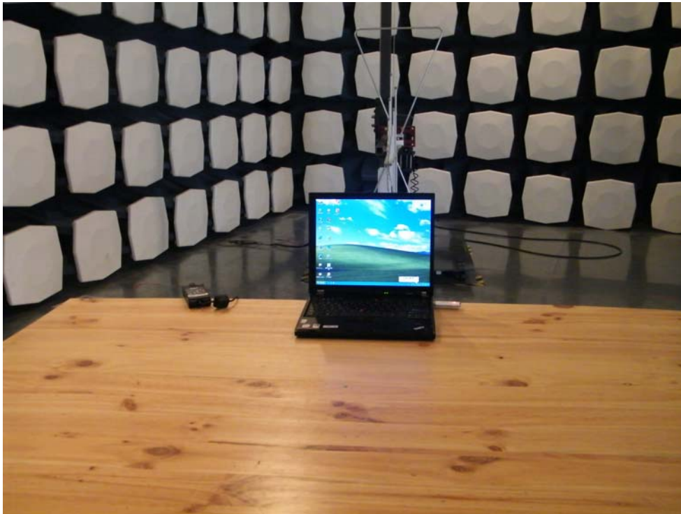
Picture 2 Radiated Emission Test Setup
