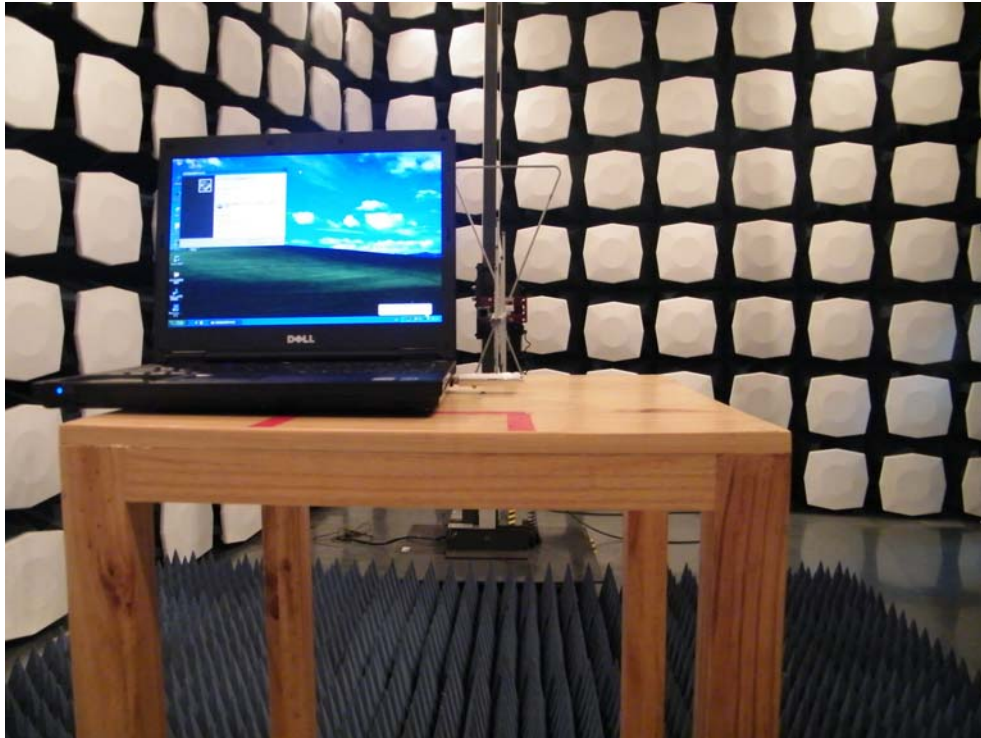
Picture 2: Radiated Spurious Emissions Test setup
