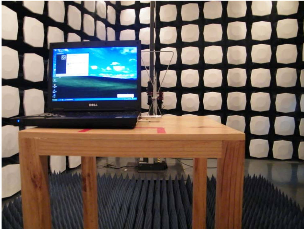
Picture 2: Radiated Spurious Emissions Test setup
