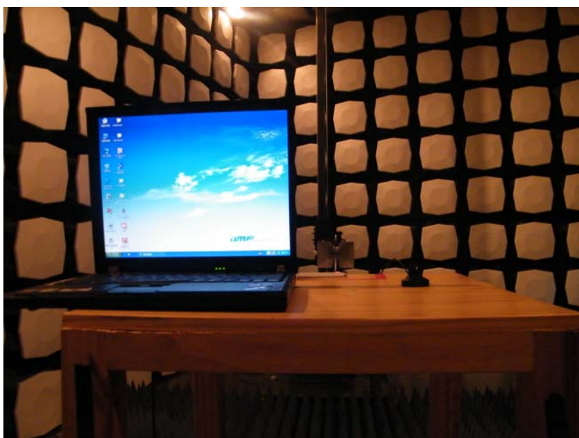
Picture 2: Radiated Spurious Emissions Test setup
