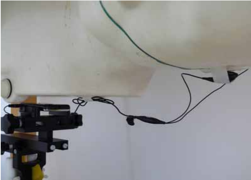
Picture 13: Body with the Earphone, towards ground, the distance from handset to the bottom of the Phantom is 15mm)
