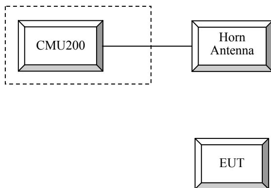
**Block Diagram of Test Setup**
