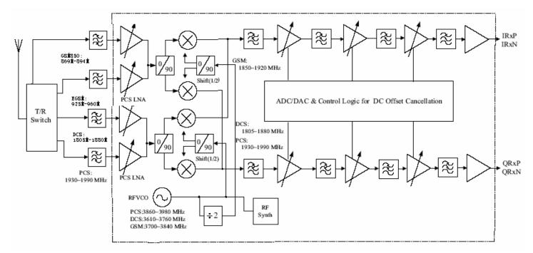
The Receiver structure in SKY77517 is a very-low IF solution. More than 100DB gain, more than 110DB control range. And by the way, all of the DC-offset canceling processes are done within chip. we do not have to care about that.
