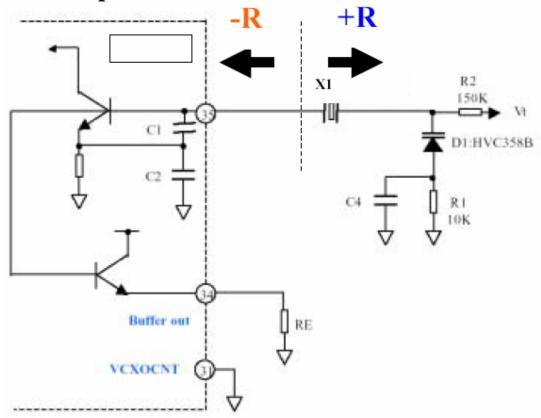
MT6139 procides a VCXO function. With that function, we can build a reference clock generation circuits as shown in the above graph. This means that the VCTCXO module is not necessary for clock application. And only one crystal with 8ppm tolerance and one varactor are enough.
