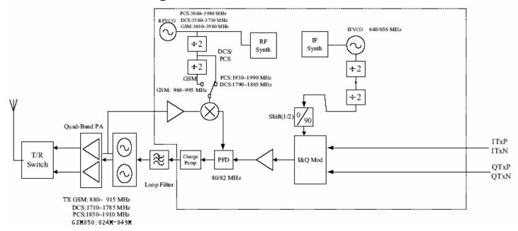
The frequency ranges of the synthesizer for TX mode are
