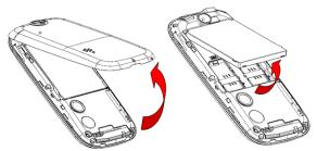
When inserting the battery, insert the metal teeth at the top of the battery into corresponding slot of the mobile phone, and then press the battery down to insert the battery in place. The battery must be correctly inserted before powering on.
