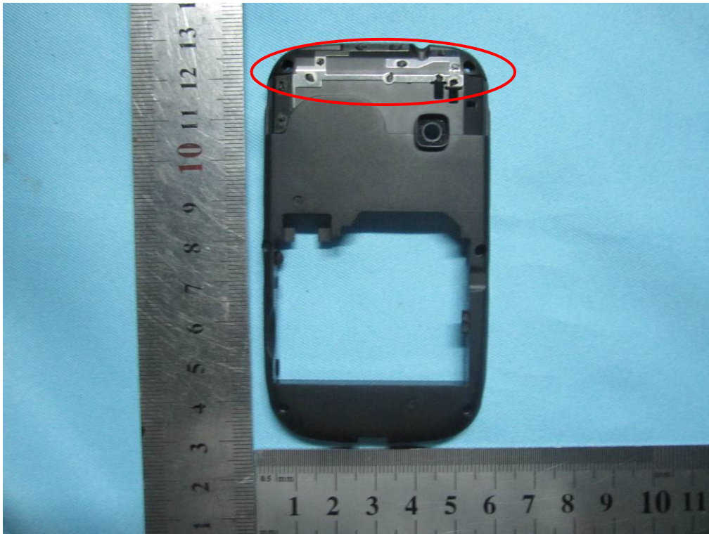
GSM / PCS Antenna View
