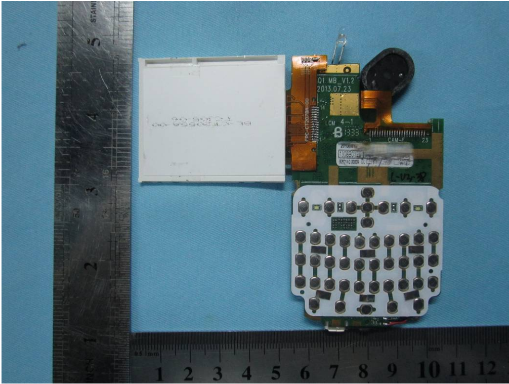
Mainboard Uncover - Top View
