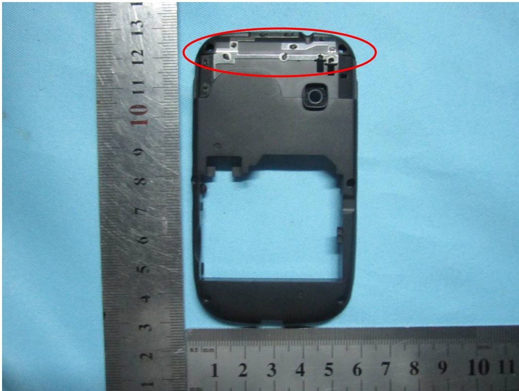
GSM / PCS Antenna View
