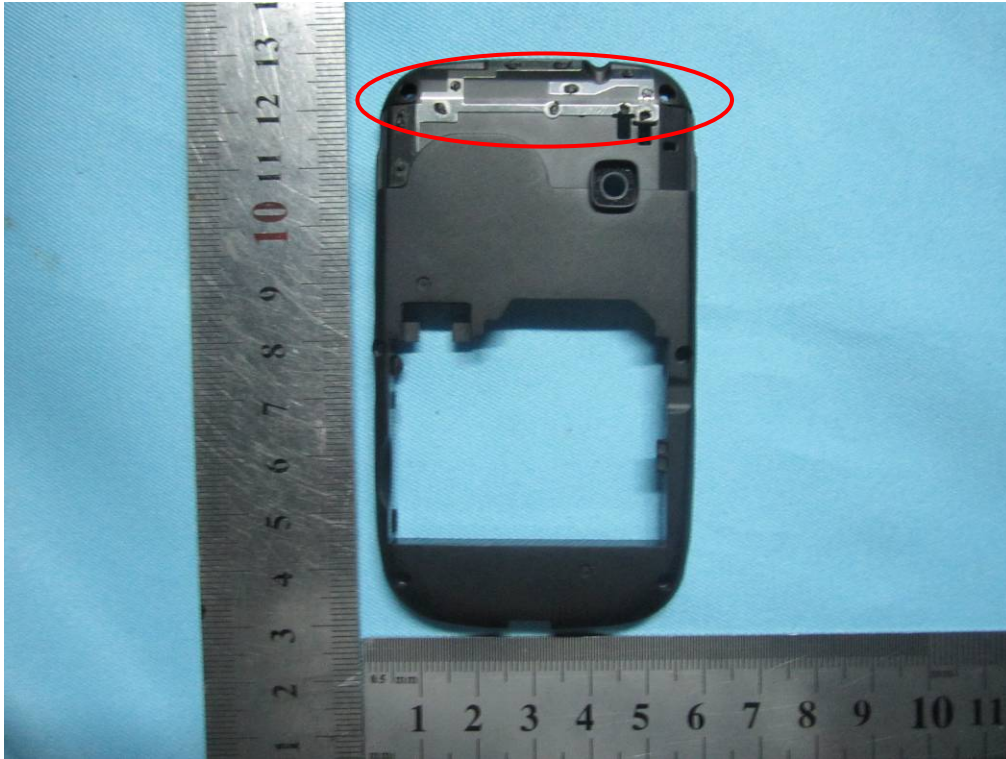
GSM / PCS Antenna View
