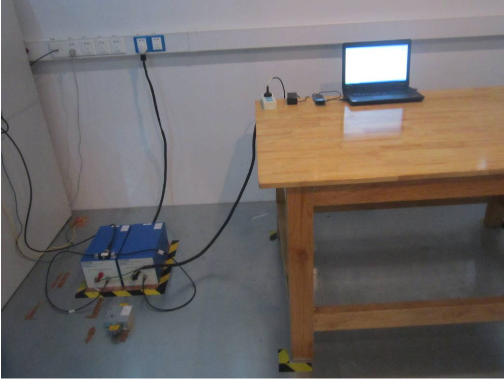
Conducted Emissions Test Setup Front View
