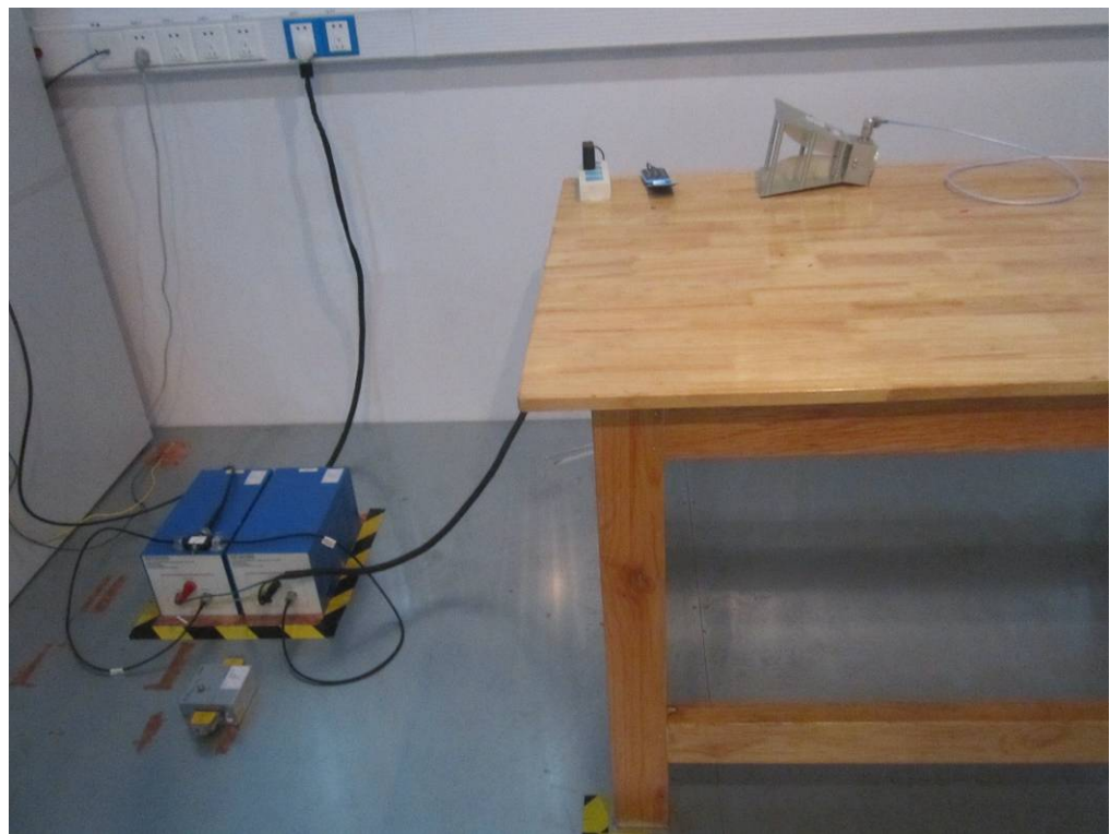
Conducted Emissions Test Setup Front View
