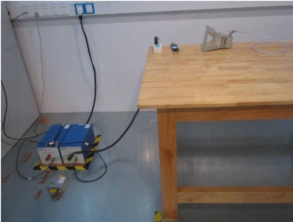
Conducted Emissions Test Setup Front View
