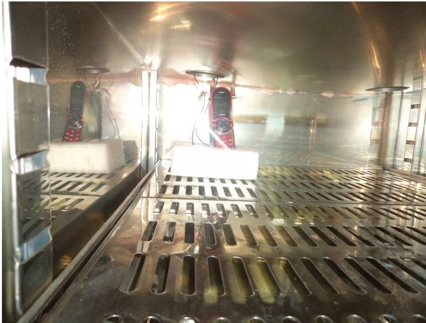
Frequency Stability Test View
