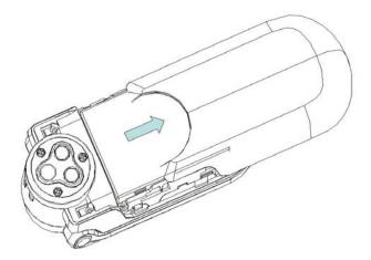
2. Aim the metal terminals of the battery at those in the battery compartment and then push down and into it.
